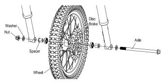
**2** Slide axle through fork, spacer and wheel hub. When axle passes through the other side of the wheel hub, add the other spacer and slide though the fork. Secure with washer and nut.
