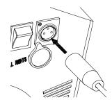
**2** Turn **OFF** power switch before charging. Plug charger into the charger port on the electric motor bike.
