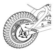
1 Loosen screw and remove chain guard.
