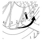
**2** Start with spoke closest to the tire valve stem and tighten each nipple, in sequence, exactly 1/4 to 1/2 turn. A single 1/4 to 1/2 turn may not be enough to bring the spokes into proper tension. Continue tightening all spokes no more than 1/2 turn in sequence until all spokes are tight.
