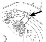
2 If the brake has too much slack, loosen the rear anchor bolt with a 5mm Allen wrench and pull the brake wire tighter. The distance of the brake wire between the end of the cable and the anchor bolt should be between 37mm and 44mm.
