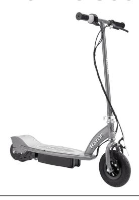
**NOTE:** The unit must be traveling up to 3mph (5kmh) before motor will engage. Kick start up to 3mph (5kmh) while applying the throttle to engage motor.
