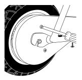
**1** With a Phillips screwdriver, remove the screws that secure the chainguard. Remove chainguard.
