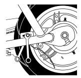
**7** Tighten the brake housing anchor securely.
