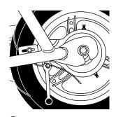
**2** With a 10mm wrench, loosen the brake cable anchor and disconnect the brake cable.
