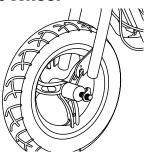
**2** Insert the wheel into the front fork with the lock washers on the outside of the fork.
