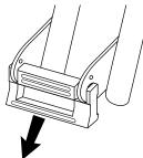
**1** Remove the packing material from the front fork.
