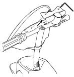
**1** Loosen the two hexagonal bolts with the 3mm hexagonal wrench and remove the plastic handlebar cover.
