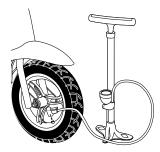
**1** Using a bicycle style tire pump equipped for a Schrader-type valve, inflate the front tire to the PSI indicated on the sidewall of the tire.
