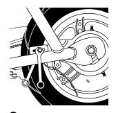
**3** With two 8mm wrenches, loosen the brake housing anchor and disconnect. Keep the spacer and washers together.
