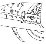
**2** If the brake lever adjuster is threaded outward and the brake still has too much slack, use the rear brake adjuster for additional adjustment.
