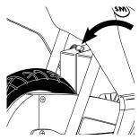
**2** Locate fuse cover on top of battery assembly through the rear fender.
