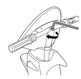
**3** Tighten down the hexagonal bolt with the 6mm hexagonal wrench
