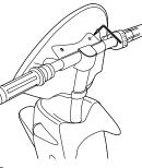
**5** Secure the two hexagonal bolts with the 3mm hexagonal wrench.
