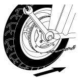
**4** With two 17mm wrenches, loosen the axle nuts. Push the wheel forward in the slots to loosen the chain.
