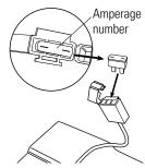
**4** Remove the fuse and replace with a new one of equal amperage.
