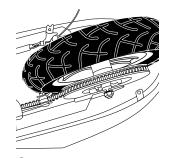
**6** Install the new chain or wheel by slipping the chain around the axle. Slide the axle into the slots on the frame. Slide the wheel forward and maneuver the chain onto the rear sprocket, front sprocket and chain tensioner. Tighten the axle nuts.
