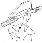
**2** Insert handlebar assembly into the fork until it stops. Raise to desired height, keeping the stem and fairing aligned within the red arrows of the safety zone.
